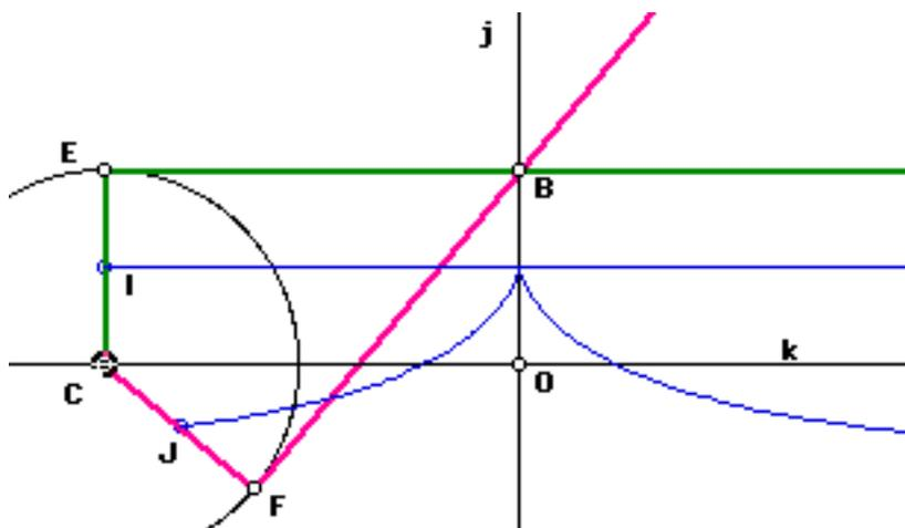
Newton showed that cissoid of Diocles can be generated by sliding a right triangle. This method also easily proves the tangent construction.
