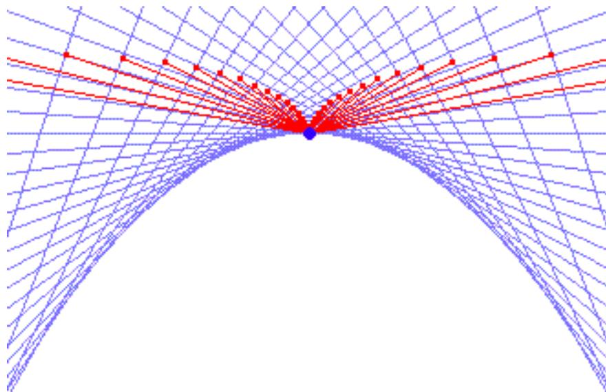
The pedal of a parabola with respect to its vertex is the cissoid of Diocles. (and then by definition, the negative pedal of a cissoid of Diocles with respect to its cusp is a parabola.)
