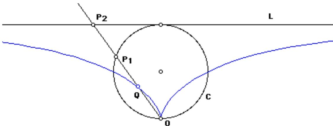
The Cissoïd of Diocles is a special case of the general cissoïd. It is a cissoïd of a circle and a line tangent to the circle with respect to a point on the circle opposite to the tangent point. Here is a step-by-step description of the construction:
