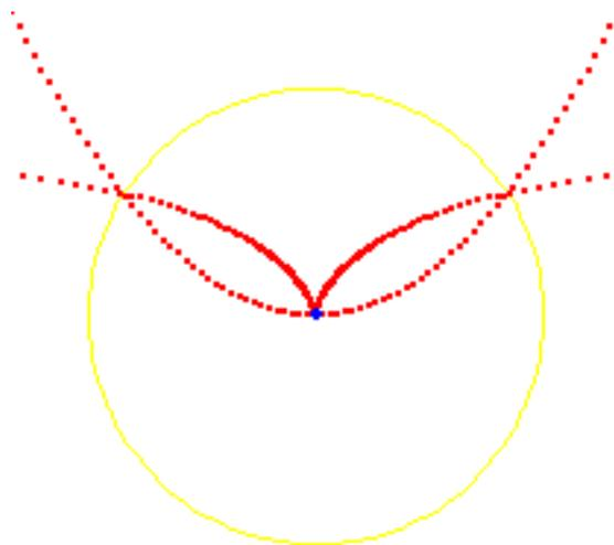
The inversion of a cissoid of Diocles at cusp is a parabola.
