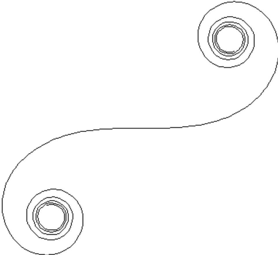
The Clothoid is also called Euler spiral and Spiral of Cornu, is a curve whose curvature is equal to its arclength. It has the parametric formula:
